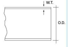
The pipe is plain and for solvent weld jointing. Full details of dimensions of all sizes, minimum wall thickness and pipe lengths are given in the following tables.
